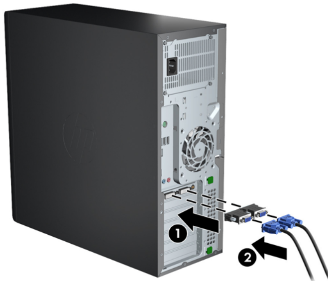
Figure 3-4 Connecting the cables to the workstation
