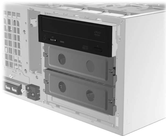
Figure 3-9 Reinstalling the optical drive
